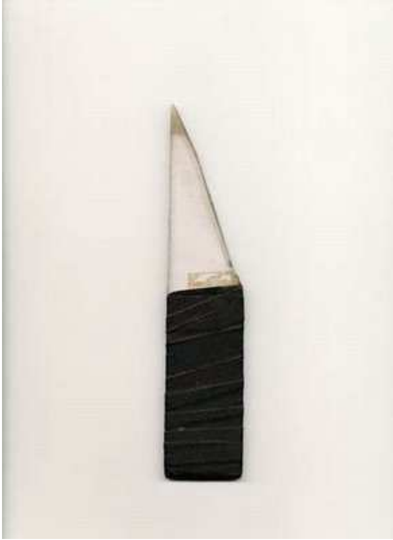
Materials: Shard of plexiglas; handle wrapped with electrical tape.
