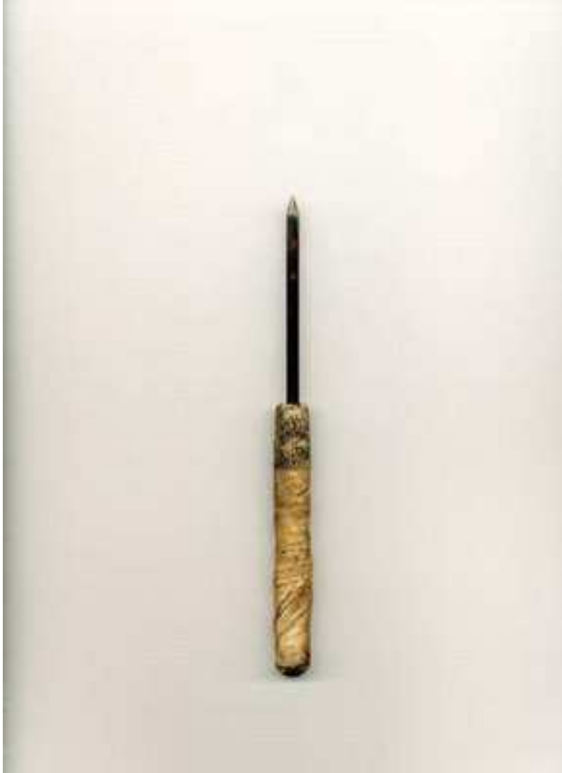
Materials: Steel rod; handle wrapped with boxing tape.
